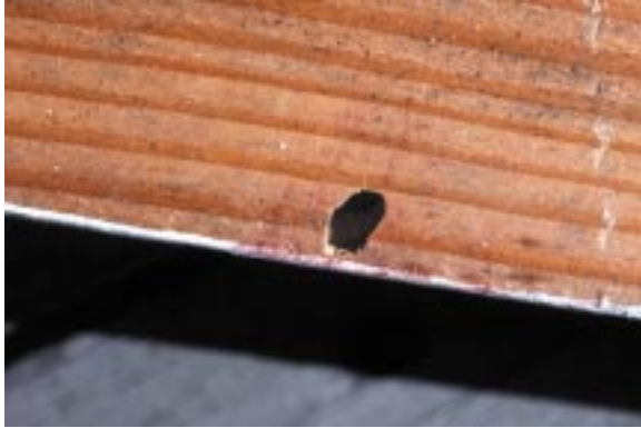
Fig. 5a. Buprestid beetle exit hole.
